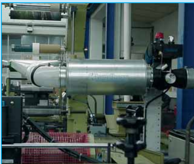
GR140MS Matrix connected to a machine with webs up to 410 mm wide.
