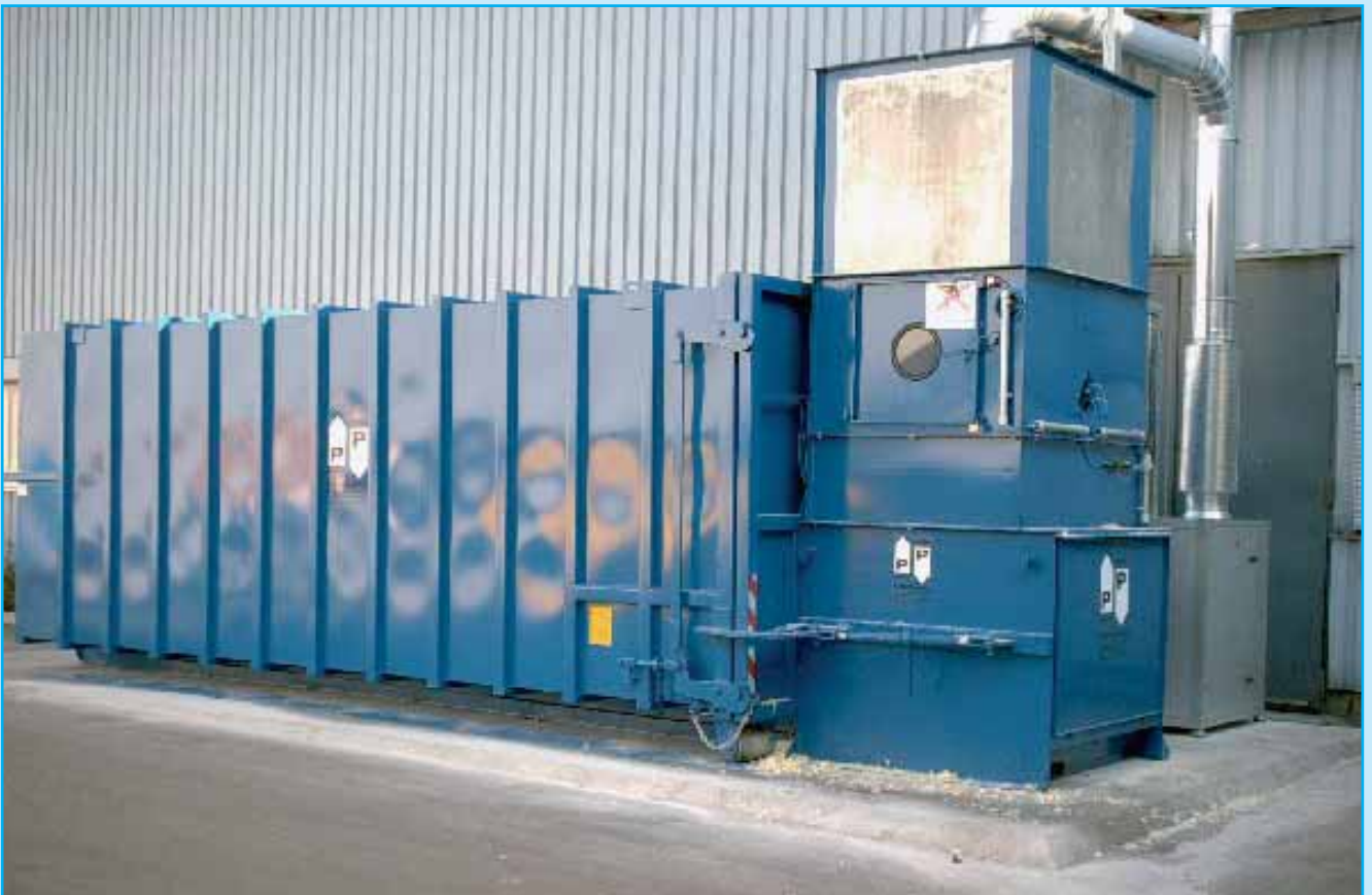
Main extraction from granulating plant connected to automatic label printing machines The granulated paper, adhesive coated waste is collected in a compactor.
