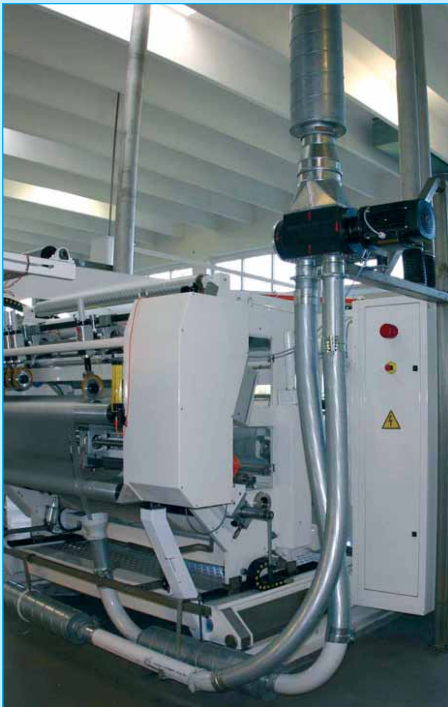
Granulator mounted on take-up for extruding line
